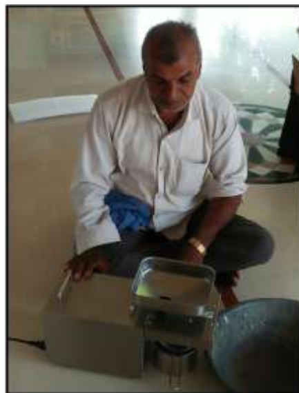
Farmer with his own manufactured neem oil extruder
